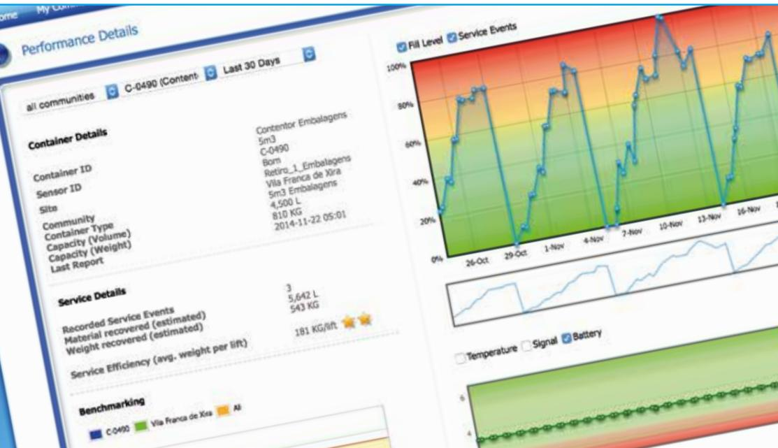
The fill level management and route planning SOTKIS is a system that uses an ultrasonic sensor and a web portal to provide information on the state of filling in each container.
