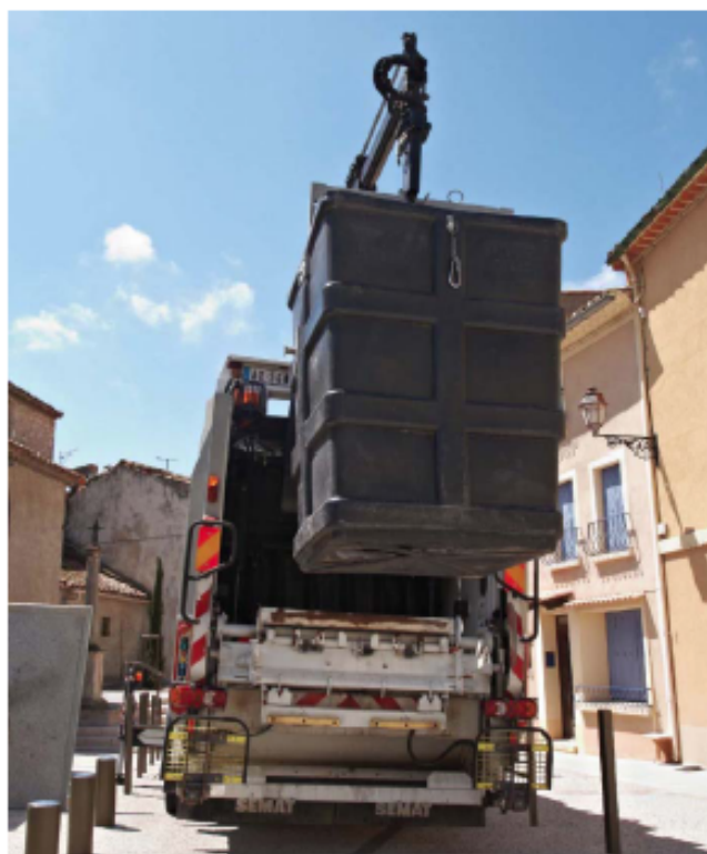
The container is dropped down to the ground in front of the RCV loading hopper...
